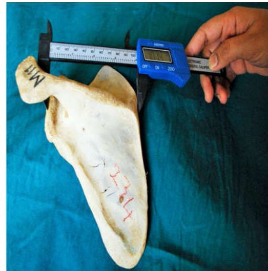
Fig. 3: Showing measurement of scapular breadth with digital vernier caliper
